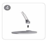
Take the Stand Connector out of the Stand by pulling it in the direction of the arrow as shown in the figure.
